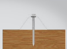
12 x 65mm Type 17 hex head screw or 12 x 65mm TS self drilling screw
